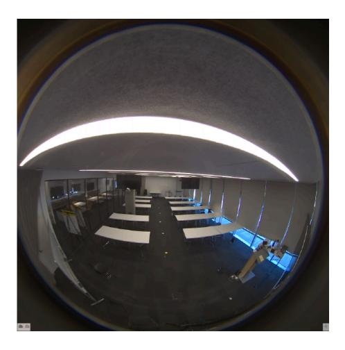
Furthermore, the camera's computer vision analytics function on training algorithms based on a top-down view of its surroundings. Orientations differing from this model will limit the performance of the camera's analytics. Therefore, it is not recommended to install the MV32 perpendicular to the ground.
